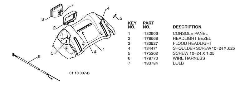
**NOTE:** All component dimensions given in U.S. inches. 1 inch = 25.4 mm **IMPORTANT:** Use only Original Equipment Manufacturer (O.E.M.) replacement parts. Failure to do so could be hazardous, damage your snow thrower and void your warranty.
